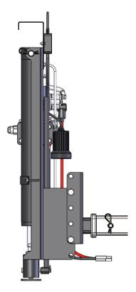
7. To attach motor cover, slide cover from top over motor (opening to frame). Remove the bolt on the right side of the frame and be sure to support the hydraulic motor. Place the motor cover in front of the motor mount, line up the holes, and re-bolt the cover to the frame. Move to the left side of the frame and remove the top bolt. Place the cover over motor mount, line up the holes and re-bolt. The cover is fairly flexible which will allow you to bolt one side at a time.
